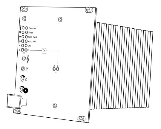
The 25 / 50 W amplifier as well as the 100 W amplifier are designed in 100 Volt technology. The very compact amplifiers are used to amplify the power of Neumann Elektronik ELA, DS-6 and MDK systems, and also offer the possibility of connection to all voice communication centres with analogue interfaces.
